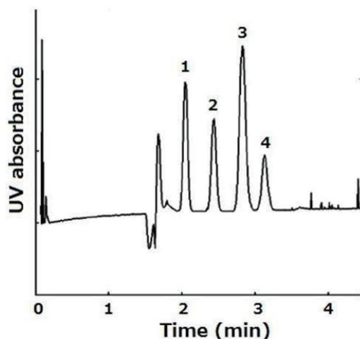
**Fig. 8.** Electrochromatogram of microdialysate sample-spiked with 25  $\mu\text{g/ml}$  of caffeine and its two metabolites. Conditions: mobile phase, 4.0 mM citrate buffer-methanol (20:80, v/v %). Other conditions as in Fig. 7. Peaks: 1, 1-methylxanthine; 2, 1,7-dimethylxanthine; 3, pentoxifylline (E.S.); 4, caffeine. Reproduced from ref. [21] with permission.
