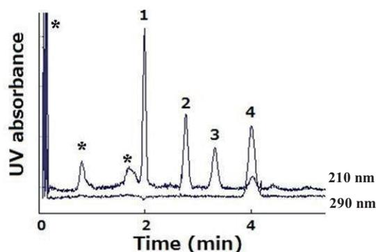
**Fig. 7.** Electrochromatogram of the serum sample spiked with barbiturates standards. Stationary phase, NAIP; column, 340 mm (packed length 90 mm) x 75  $\mu$ m i.d.; mobile phase: 1.0 mM citrate buffer (pH5.0)-methanol (60:40, v/v %). Other conditions as in Fig. 2. Peaks: 1, barbital; 2, phenobarbital; 3, secobarbital; 4, thiopental; \*, Peaks for intrinsic components in serum. Reproduced from ref. [20] with permission.
