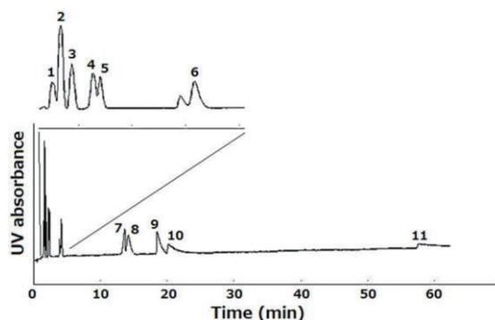
**Fig. 5.** Electrochromatographic separation of nucleosides and nucleic acid bases on SNAIP. Mobile phase, 10 mM phosphate buffer (pH 5.0)-methanol (90:10, v/v %); applied voltage, 15 kV. Other conditions as in Fig. 2. Peaks: 1, uridine; 2, uracil; 3, thymidine; 4, thymine; 5, inosine; 6, guanosine; 7, adenosine; 8, cytidine; 9, guanine; 10, cytosine; 11, adenine. Reproduced from ref. [14] with permission.
