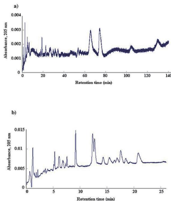
**Fig. 6.** Effect of buffer concentration on the separation of tryptic digests of cytochrome *c*. Mobile phase, phosphate buffer (pH 3.8)-methanol (60:40, v/v %) at different buffer concentrations: (a) 20 mM (27  $\mu$ A); (b) 50 mM (95  $\mu$ A); applied voltage, 20 kV. Other conditions as in Fig. 2. Reproduced from ref. [18] with permission.
