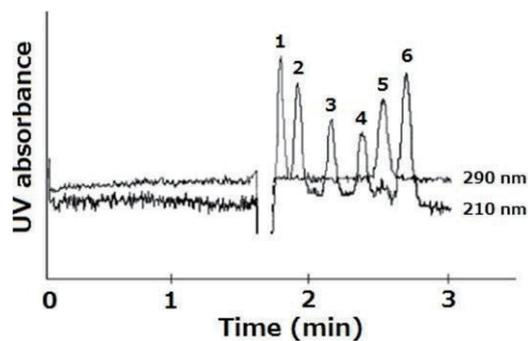
**Fig. 3.** Electrochromatogram of barbiturates with SNAIP. Mobilephase: 5 mM phosphate (pH 3.8)-methanol (60:40, v/v %). Other conditions as in Fig. 2. Peaks: 1, thiourea; 2, barbital; 3, amobarbital; 4, secobarbital; 5, thiopental; 6, phenobarbital. Reproduced from ref. [12] with permission.
