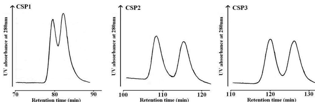
**Fig. 9.** Typical chromatographic separations of *R/S*-warfarin with CSP1-3. Mobile phase: 0.5M sodium perchlorate (pH 2.0)-acetonitrile (77:23, v/v %). Reproduced from ref. [36] with permission.
