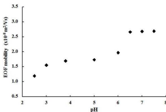
Fig. 2. Dependence of EOF mobility with SNAIP on the pH of mobilephase. Column, total length 370 mm (packed length 90 mm)  $\times 75 \mu\text{m}$  i.d.; mobile phase, 5 mM phosphate-methanol(60:40, v/v) at different pH values; applied voltage, 20 kV; temperature, 18 °C. Reproduced from ref. [12] with permission.
