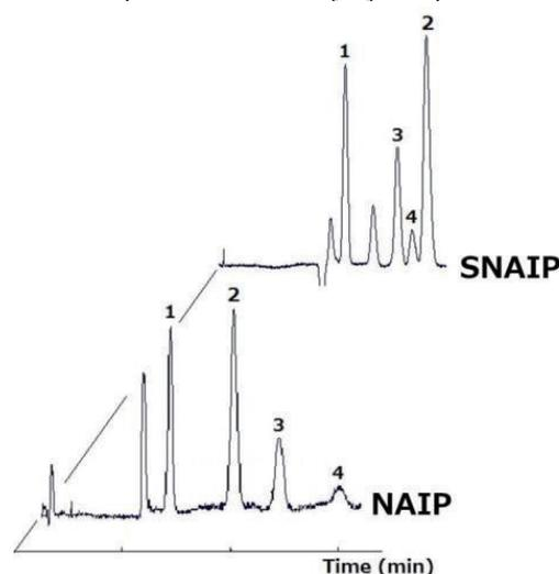
**Fig. 4.** Electrochromatographic separation of barbiturates with SNAIP and NAIP. Stationary phase, SNAIP; mobilephase, 5 mM phosphate(pH 3.8)-methanol (60:40, v/v %); applied voltage, 10 kV. Stationary phase, NAIP; mobile phase, 1 mM citrate (pH5.0)-methanol (60:40, v/v %); applied voltage, 20 kV. Other conditions as in Fig. 2. Peaks: 1, thiourea; 2, phenobarbital; 3, secobarbital; 4, thiopental. Reproduced from ref. [12] with permission.
