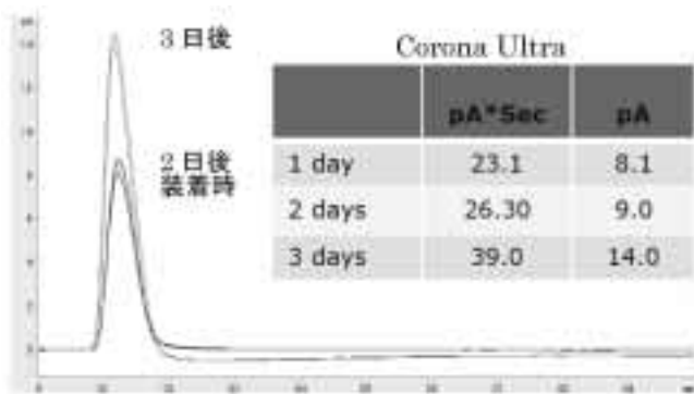
Figure 7. Extraction Peak from AC Cartridge by CORONA CAD.
