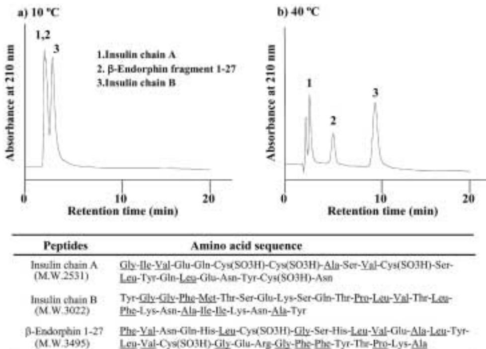
**Figure 9.** Chromatograms of peptides using poly (NIPAAm-*co*-BMA 5%) modified column. Hydrophobic amino acids were indicated underline. HPLC conditions: flow rate, 1.0 mL/min; detection, UV at 210 nm; eluent, 0.9 w/v% NaCl aqueous solution; injection volume, 10 $\mu$ L; column, PNIPAAm-*co*-BMA 5% terminally modified Silica.
