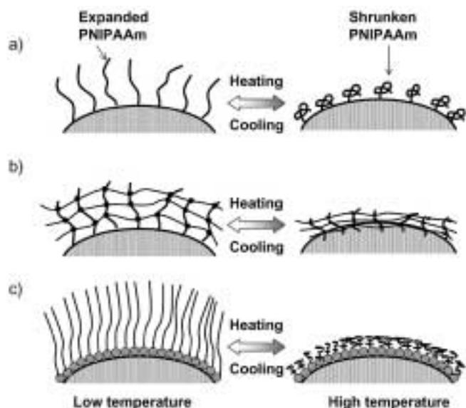
**Figure 1.** Schematic illustration of a various grafting methods of PNIPAAm to the silica surface; a) terminally modified; b) hydrogel modified; c) polymer brush by ATRP.
