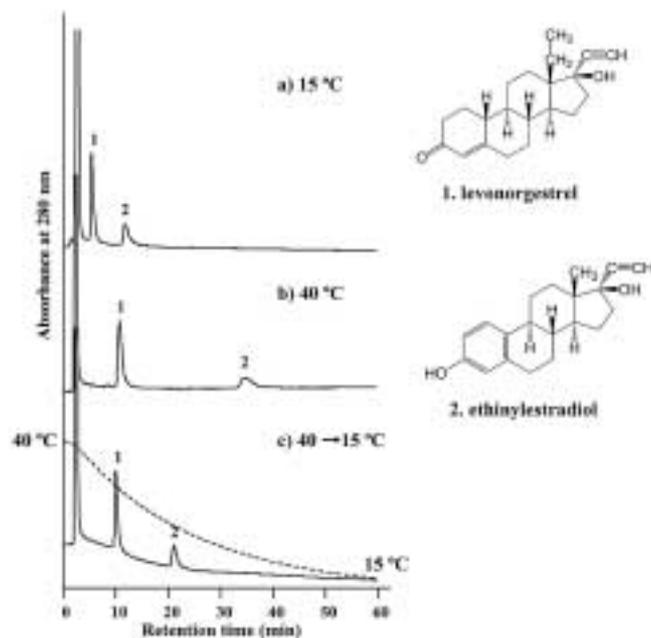
**Figure 8.** Effects of temperature changes on the retention times of levonorgestrel and ethinylestradiol. HPLC conditions: flow rate, 1.0 mL/min; eluent, water; detection, UV at 280 nm; column, PNIPAAm-modified column; temperature gradient speed, 25°C/60 min.
