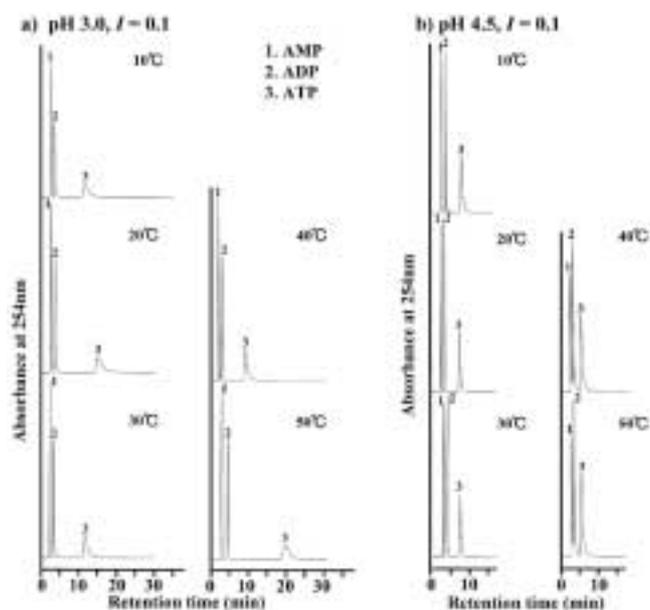
**Figure 6.** Chromatograms of adenosine nucleotides (AMP, ADP, and ATP) on poly (NIPAAm-*co*-BMA-*co*-DMA-PAAm) modified silica column. HPLC conditions: flow rate, 1.0 mL/min; eluent, phosphate/citrate buffer.
