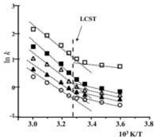
**Figure 5.** The effects of temperature on the retention factor of the steroids on the PNIPAAm-modified column. HPLC conditions are the same as those in Figure 3. Samples:  $\circ$ , hydrocortisone;  $\blacktriangle$ , prednisolone;  $\triangle$ , dexamethasone;  $\blacksquare$ , hydrocortisone acetate;  $\square$ , testosterone.
