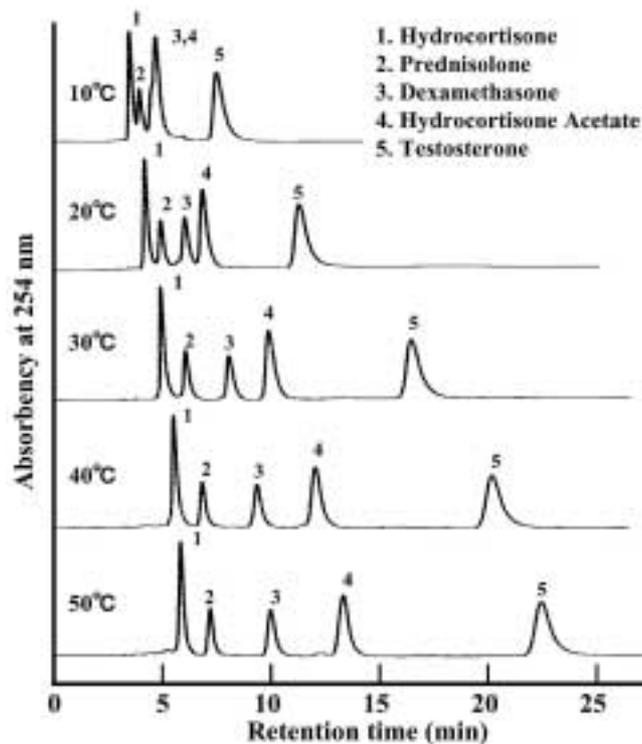
**Figure 3.** Temperature-dependent retention profile of the steroids using water as a mobile phase. HPLC conditions: flow rate, 1.0 mL/min; detection, UV at 254 nm; eluent, MilliQ-water; injection volume, 20  $\mu$ L; column, PNIPAAm-co-BMA 5% terminally modified silica (5  $\mu$ m, 4.6 mm I.D.  $\times$  150 mm).
