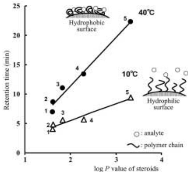
**Figure 4.** Effects of the log  $P$  value of steroids on the retention times. Column, PNIPAAm-modified column (5 $\mu$ m, 4.6 mm I.D.  $\times$  150 mm); samples: 1, hydrocortisone; 2, prednisolone; 3, dexamethasone; 4, hydrocortisone acetate; 5, testosterone. HPLC conditions; detection, UV at 254 nm; eluent, pure water; flow rate, 1.0 mL/min.
