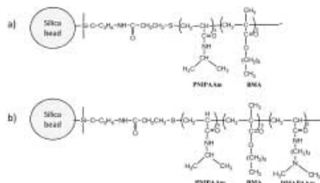
**Figure 2.** The structural formulas of copolymer modified silica; a) PNIPAAm-co-BMA modified silica, b) poly (NIPAAm-co-BMA-co-DMAPAAm) modified silica.
