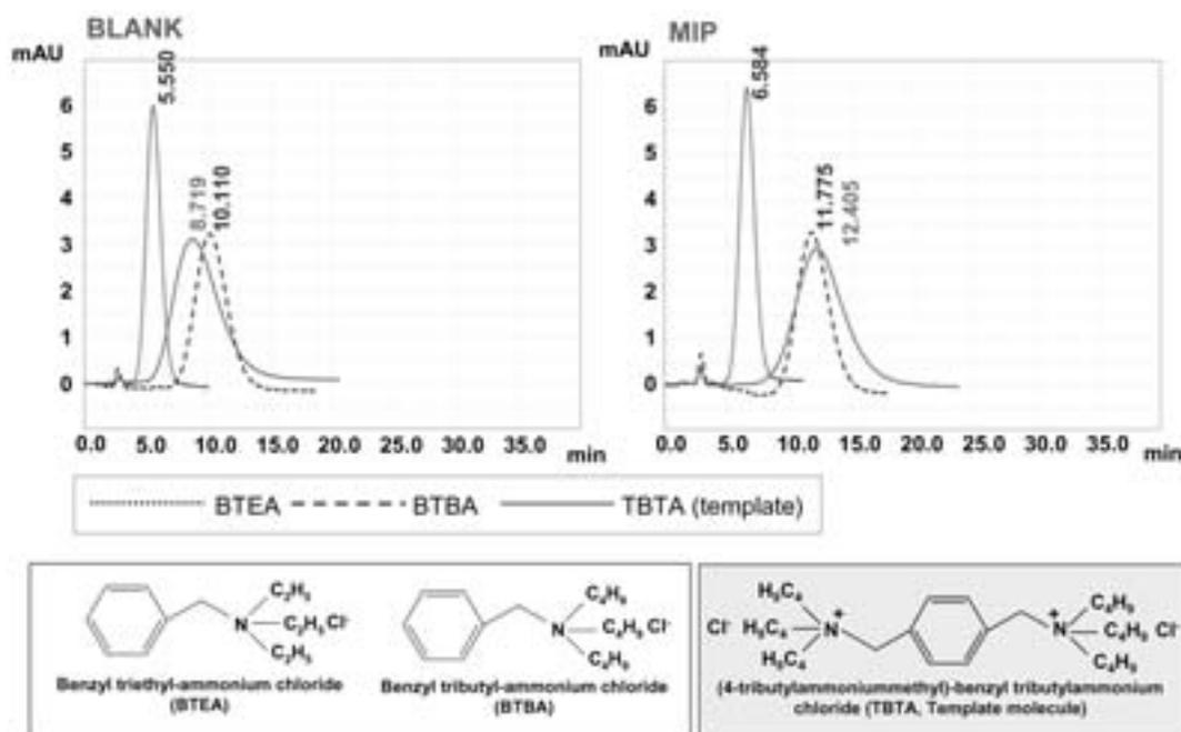
**Figure 6.** Chromatograms of the ionic solutes on Blank and MIP. LC conditions: Mobile phase; 0.1 M NaCl aqueous, Flow rate; 0.5 ml min<sup>-1</sup>, Column size; 100 mm \* 4.6 mm i.d., Temperature; 30°C, Detection; Photo diode array
