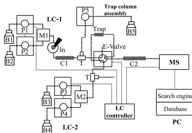
**Figure 1.** Schematic diagram of the 2 DLC–MS/MS system. The assemblies are explained in the text. B 1–5, eluents 1–5; C 1, ion–exchange column; C 2, reversed phase column; D, drain; E–Valve, electric valve; In, injector; M, dynamic mixer; P 1–5, pumps 1–5; Trap, trap column; T, T connector.
