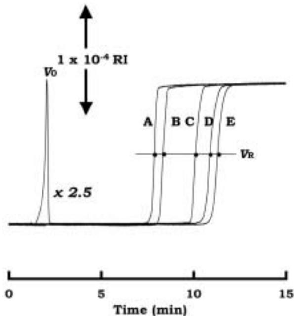
**Figure 16.** Breakthrough curves of calcinated Pia Seed 5 S-60-SIL columns with 0.75 mM tyramine-0.25 mM oxalic acid-5 mM 15-crown-5 at pH 5.0 as eluent
