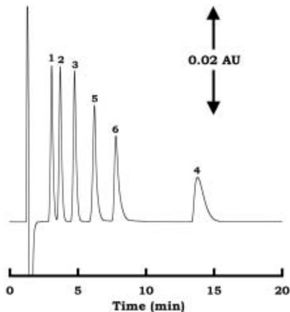
**Figure 12.** Chromatograms of mono- and divalent cations on Pia Seed–1000 column with 0.75 mM tyramine–0.25 mM oxalic acid–0.5 mM 18-crown-6 at pH 5.0 as eluent
