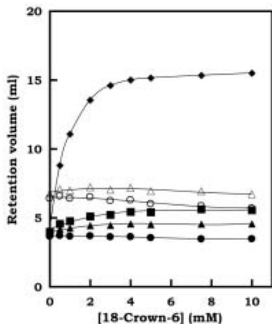
**Figure 8.** Effect of concentration of 18-crown-6 in 0.2 mM oxalic acid at pH 3.6 as eluent on retention volumes of mono- and divalent cations on Pia Seed 5S-60-SIL column
