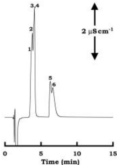
**Figure 7.** Chromatograms of mono- and divalent cations on Pia Seed 5S-60-SIL column with 0.2 mM oxalic acid at pH 3.6 as eluent
