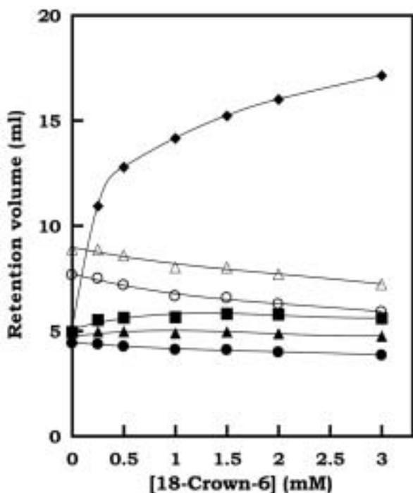
**Figure 3.** Effect of concentration of 18-crown-6 in 0.75 mM tyramine–0.25 mM oxalic acid at pH 5.0 as eluent on retention volumes of mono- and divalent cations on Pia Seed 5S–60–SIL column
