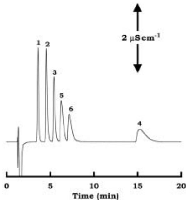
**Figure 9.** Chromatograms of mono- and divalent cations on Pia Seed 5S-60-SIL column with 0.2 mM oxalic acid–4 mM 18-crown-6 at pH 3.6 as eluent
