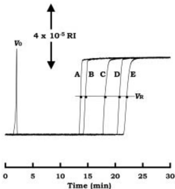
**Figure 13.** Breakthrough curves of calcinated Pia Seed 5 S-60-SIL columns with 0.75 mM tyramine-0.25 mM oxalic acid at pH 5.0 containing 1.5 mM 18-crown-6 as eluent
