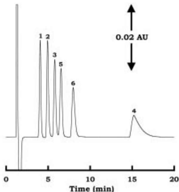
**Figure 4.** Chromatograms of mono- and divalent cations on Pia Seed 5S–60–SIL column with 0.75 mM tyramine–0.25 mM oxalic acid–1.5 mM 18-crown-6 at pH 5.0 as eluent
