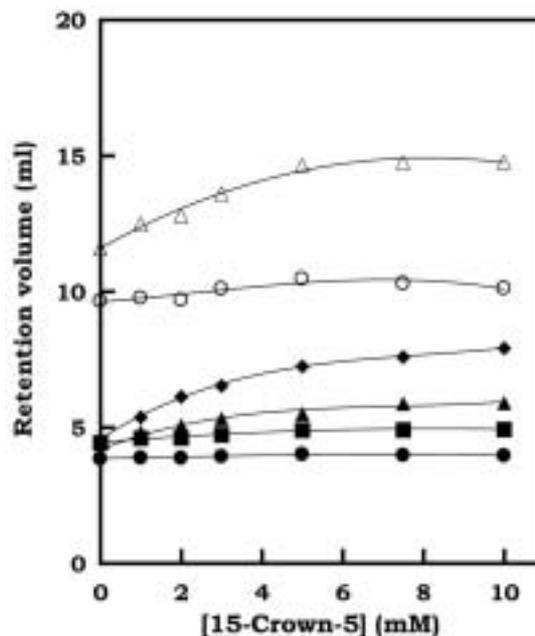
**Figure 14.** Effect of concentration of 15-crown-5 in 0.75 mM tyramine-0.25 mM oxalic acid at pH 5.0 as eluent on retention volumes of mono- and divalent cations on Pia Seed-1000 column
