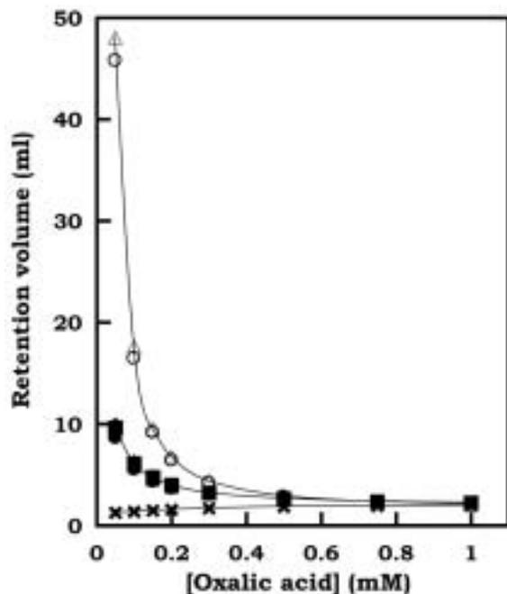
**Figure 6.** Effect of concentration of oxalic acid in eluent on retention volumes of mono- and divalent cations on Pia Seed 5S-60-SIL column
