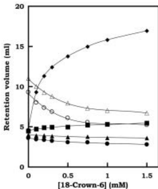
**Figure 11.** Effect of concentration of 18-crown-6 in 0.75 mM tyramine–0.25 mM oxalic acid at pH 5.0 as eluent on retention volumes of mono- and divalent cations on Pia Seed–1000 column
