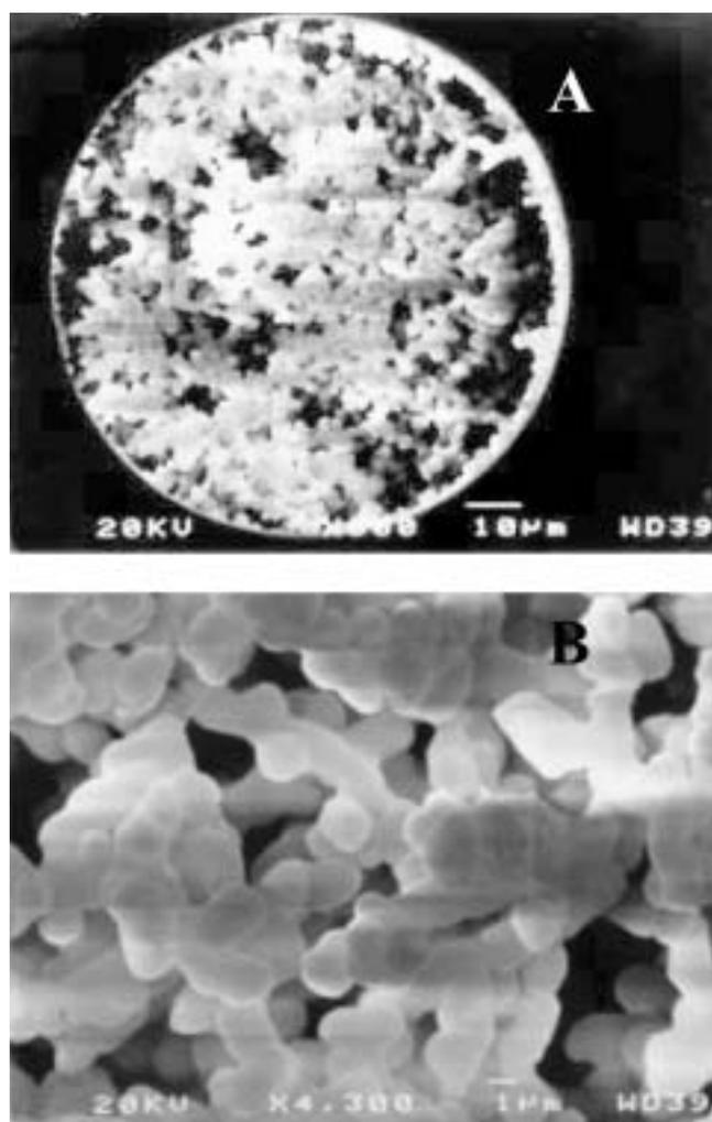
**Figure 8.** SEM photographs of sol-gel monolithic column modified with L-Phenylalaninamide: 20 kV, WD 39, and magnification (A) 800 $\times$ , (B) 4300 $\times$ . (From Ref. [33]).
