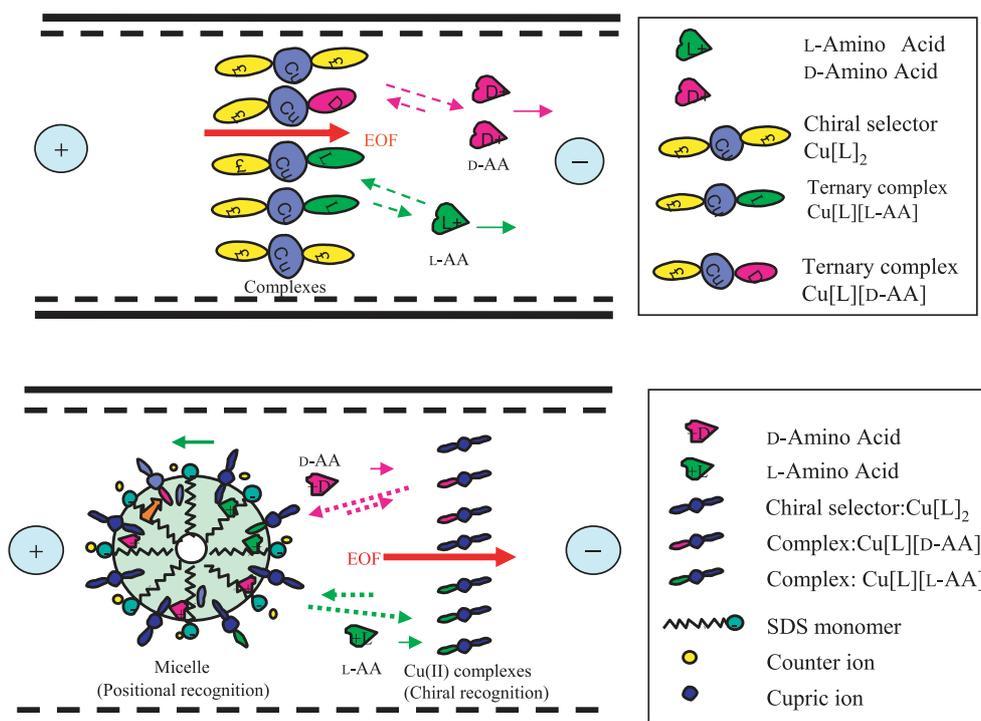
**Figure 1.** Schematic representation of proposed models of LE-CE (A, top) and LE-MEKC (B, bottom). (From Ref. [19]).
