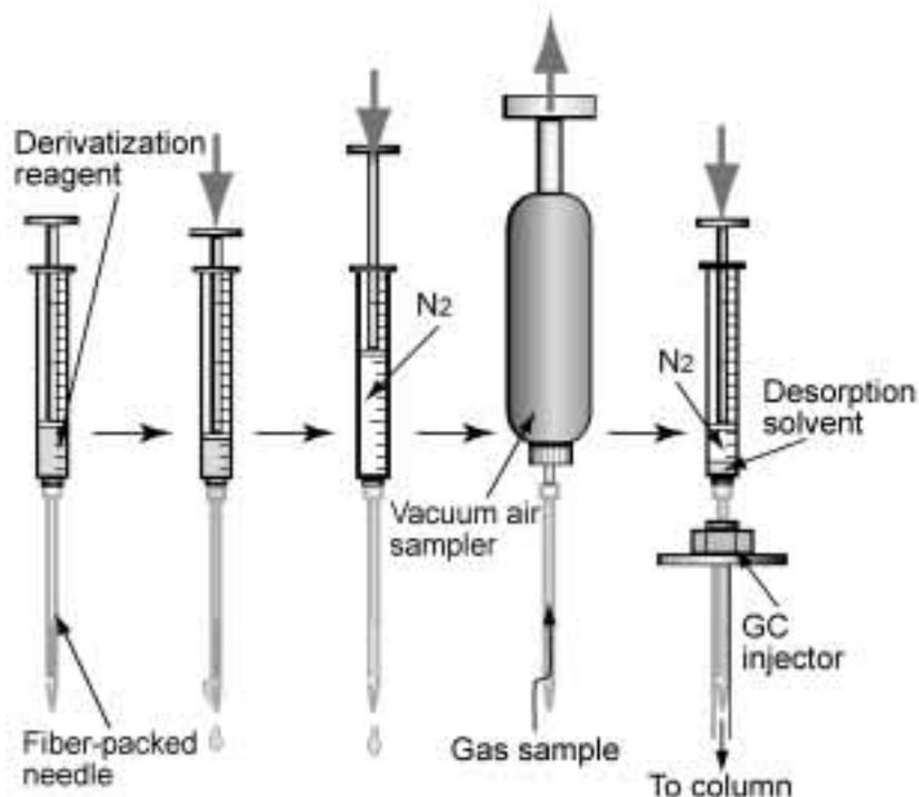
**Fig. 2** Schematic diagram of the extraction/derivatization and desorption of analytes using fiber-packed needle. Modified from Fig. 4 in reference 18 with permission.
