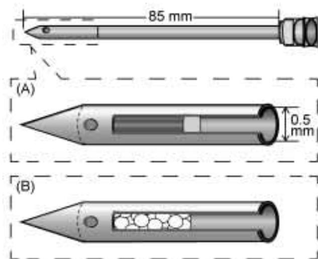
**Fig. 1** Schematic illustration of needle-type extraction devices. (A) Fiber-packed needle and (B) particle-packed needle.
