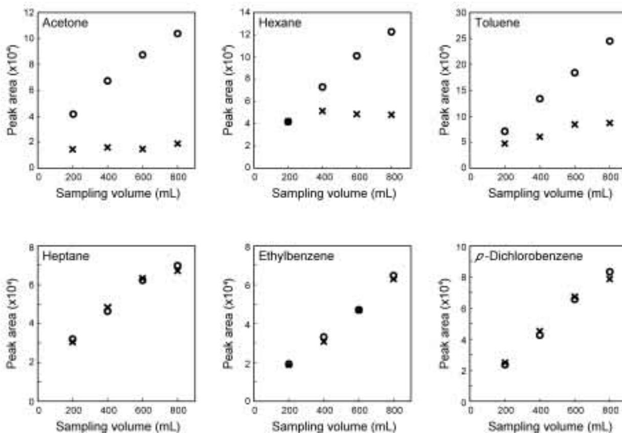
**Fig. 8** Sampling volume profiles of the DVB/AC-packed needle (circles) and DVB-packed needle (crosses). Conditions: standard gas sample concentration, 50 ng/L; sampling rate, 20 mL/min. Modified from Fig. 5 in reference 25 with permission.
