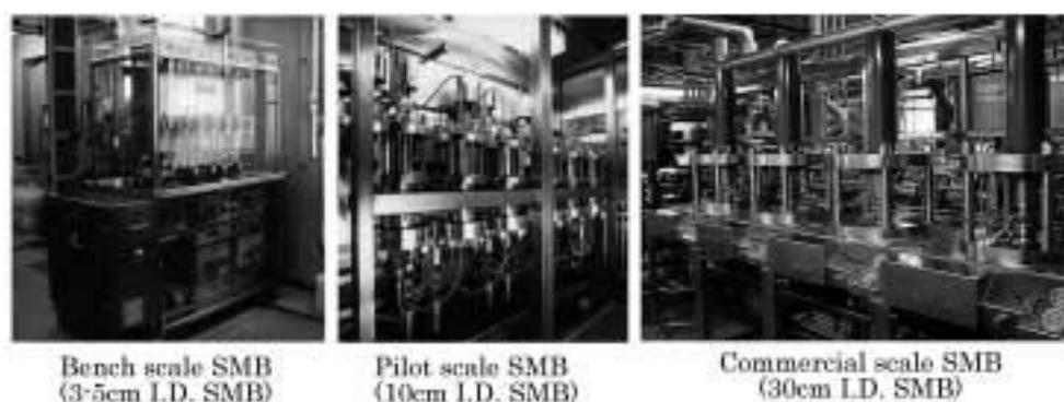
Figure 7 Daicel's lineup of the chiral SMB systems.
