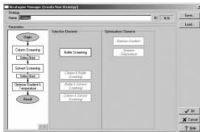
Figure 2. Building a method development strategy. In the method development strategy, shown on the left, first the stationary phase is selected, then the solvent system is selected, and finally, gradient and temperature are optimized. Buffer screening (shown in the middle column) is not a part of this strategy, but may be added if necessary.
