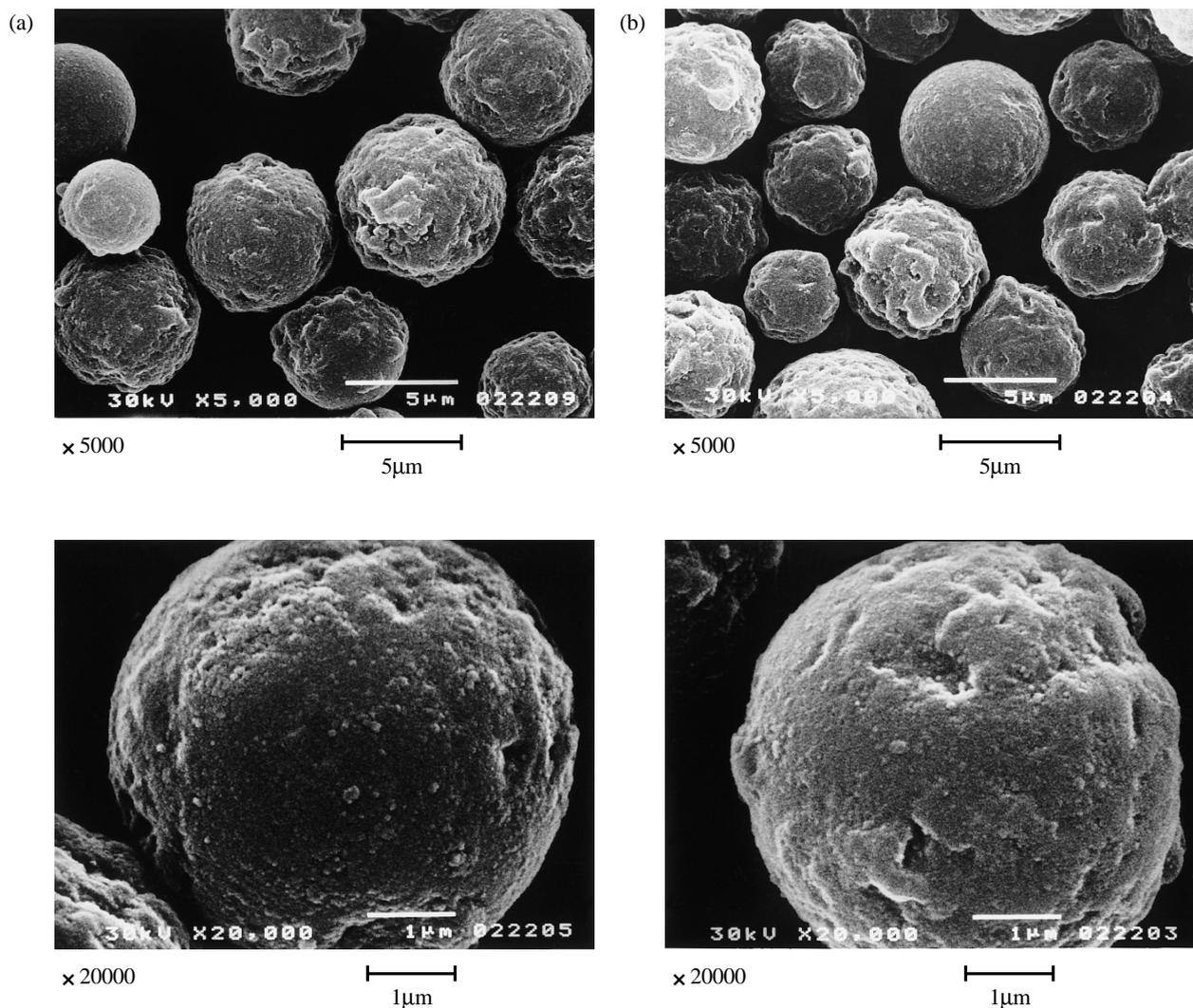
**Figure 1.** SEM of PIPAAm modified silicagel and aminopropylsilica
