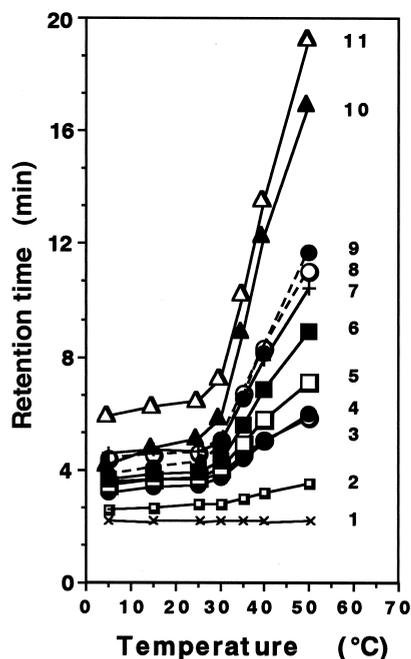
**Figure 3.** Temperature dependence of retention times of various steroids. 1: methanol, 2:benzene, 3:cortisone, 4:hydrocortisone, 5: prednisolone, 6:dexamethasone, 7: naphthalene, 8: cortisone acetate, 9: hydrocortisone acetate, 10: estriol, 11: testosterone.
