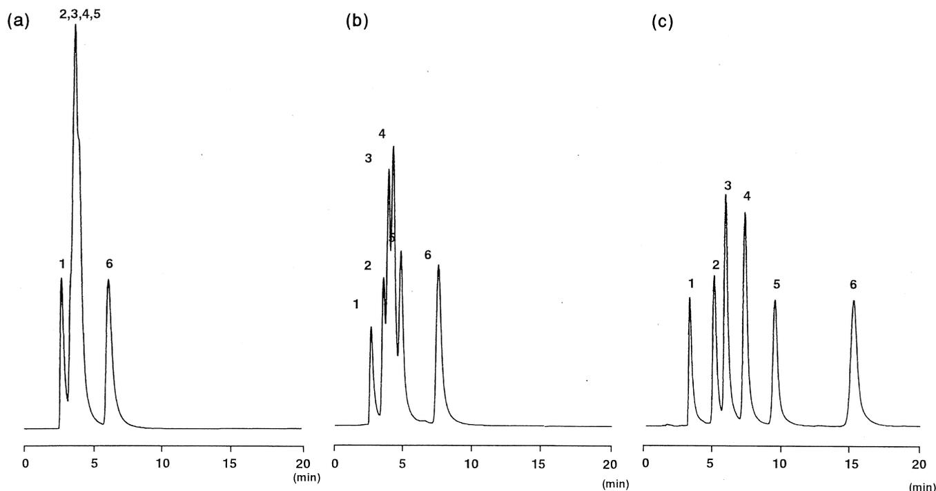
**Figure 2.** Chromatograms of a mixture of 5 steroids and benzene at various temperature. Column temperature:(a)15°C, (b) 30°C, (c) 50°C. Peak No.1: benzene, 2: hydrocortisone, 3: prednisolone, 4: dexamethasone, 5: hydrocortisone acetate, 6: testosterone. Eluent : water, flow-rate: 1.0 mL/min, detection: UV 254 nm.
